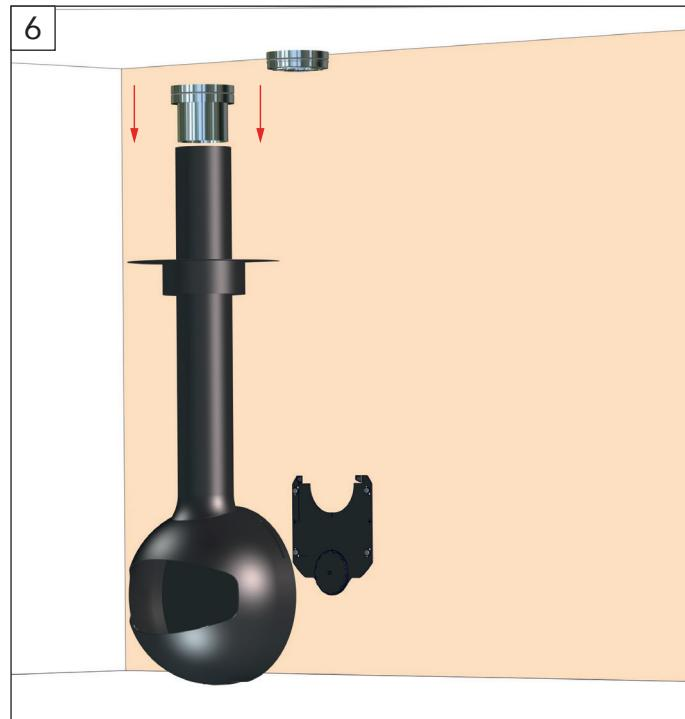
Insert the class A finishing collar with adapter into the Focus adapter.
