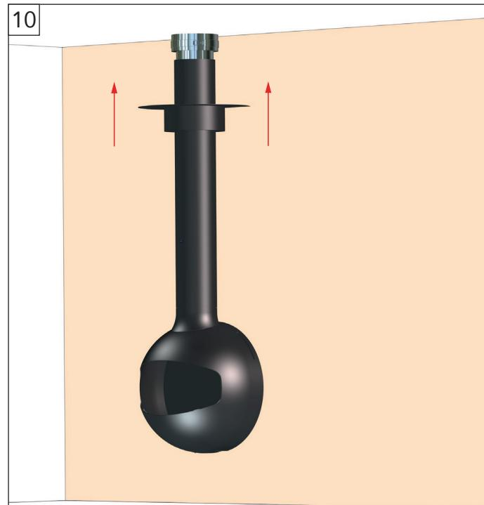
Position the conical reducer and secure it.
