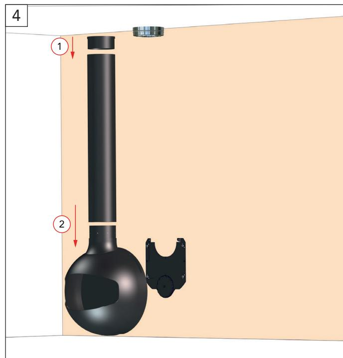
Put the 200 mm (8") Focus adapter to the end of the flue.
