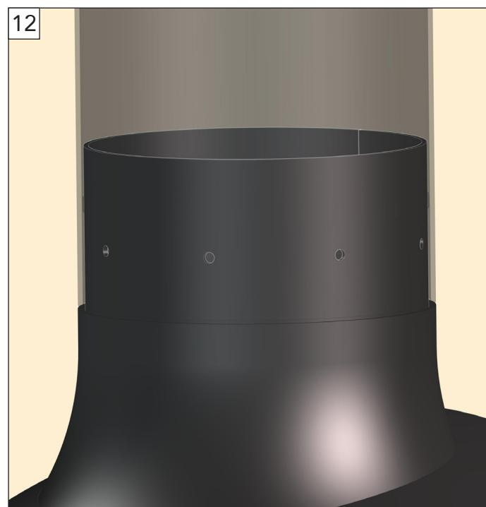
Center the duct using the 8 provided flat screws. To do this, go through the fireplace opening to access the expansion area.
